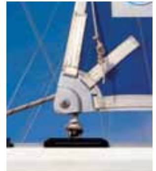
Car and track fitted on the boom
