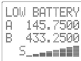
The “LOW BATTERY” indication appears when the battery voltage drops to around 4.5V and the “BATT ERR” indication appears around 3.75V. Of course these levels are only approximate and values may vary from set to set.
