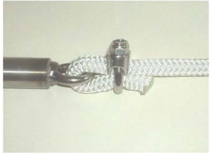
6. Attaching the tow rope to the turbine
