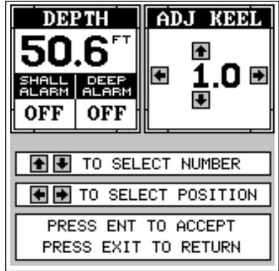
Note: Another way to use the keel offset feature is if you want to know the depth of the water below the lowest part of the boat, instead of the surface. To do this, measure the lowest part of the boat below the transducer. In this example, we'll use 3 feet. Now, using the keel offset feature, adjust the offset for a *negative* 3 feet, as shown at right.
