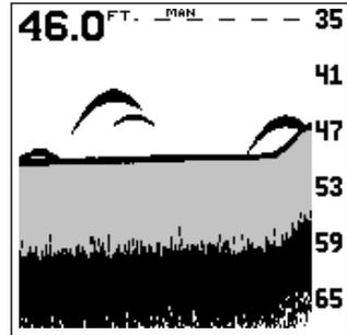
As you can see, the fish arches near the bottom are much larger and easier to see. In fact, a possible fish on the bottom shows on the enlarged screen that is not even visible on the left! Not only does this make it easier to see targets, but you can more accurately determine their depth, due to the expanded depth range.
