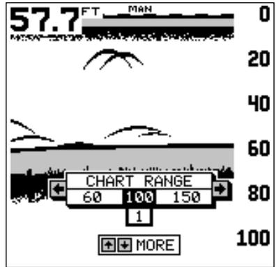
NOTE: The depth capability of the X-65 depends on the transducer installation, water and bottom conditions, and other factors.
