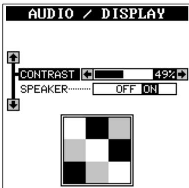
To adjust the contrast, highlight the "Contrast" menu, then use the left or right arrow key to change it. Look at the pattern at the bottom of this screen to adjust the contrast for the best sharpness.
