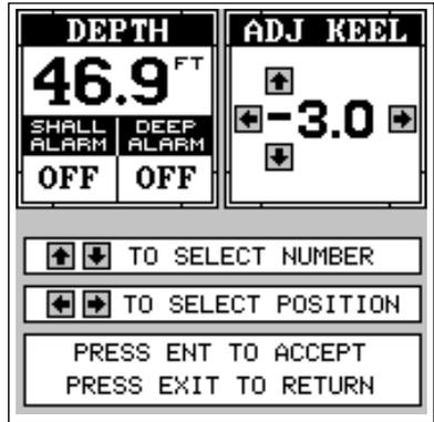
Please note that adjusting the keel offset only affects the digital depth display and all features that use the digital depth, such as the depth alarms and FishTrack. This doesn't affect the chart at all.
