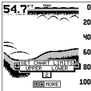
In this example, we're setting the upper limit. Use the up and down arrow keys to select the number, the right and left arrow keys to move to the next number. When the limit shows the desired depth, press the ENT key. The screen shown below appears.
