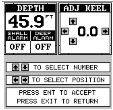
foot to the depth, since the transducer is one foot below the surface. Press the right arrow key, then the up or down arrow keys until 1.0 appears in the "Adj Keel" box, as shown at right, then press the ENT key. This immediately changes the digital depth display at the top of the screen by one foot. Press the EXIT key to erase this menu.
