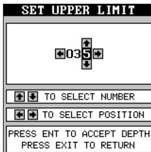
As you can see, the upper limit has changed from 0 to 35 feet. If you want to change the lower limit, repeat the above steps, press the right arrow key on the "Set Chart Limits" menu, and change the lower limit to the desired value.
