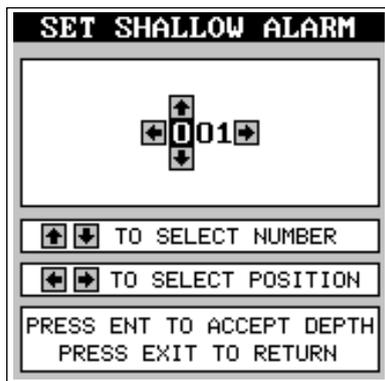
the second "0" to a "1". Next, press the right arrow key again and press the down arrow key once. This changes the "1" at the end of the number to a "0". The depth now shows 10 feet.
