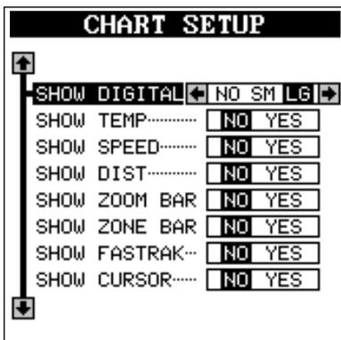
The digital depth display at the top left corner of the screen normally shows in large numbers. You can change this to smaller numbers or turn it off completely using the "Show Digital" menu at the top of this screen.
