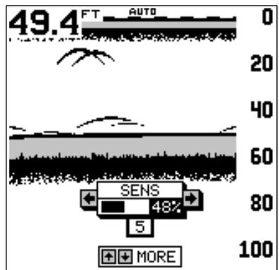
However, situations occur where it becomes necessary to increase or decrease the sensitivity. This typically happens when you wish to see more detail, so an increase in sensitivity is indicated. The procedure to adjust it is the same whether the unit is in the automatic or manual mode.
