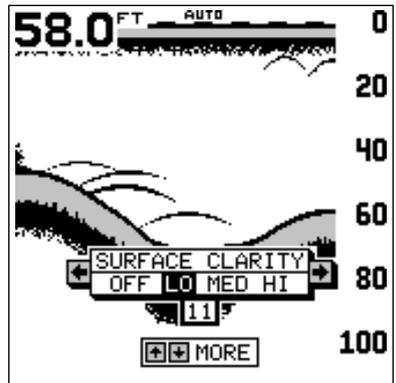
There are three levels of SCC available on the X-65: low, medium, and high. When it's turned on for the first time, the SCC level is low. To change it, press the MENU key, then press the up or down arrow keys until the "Surface Clarity" menu appears. Now use the left or right arrow keys to change it. When you're finished, press the EXIT key to erase the SCC menu.
