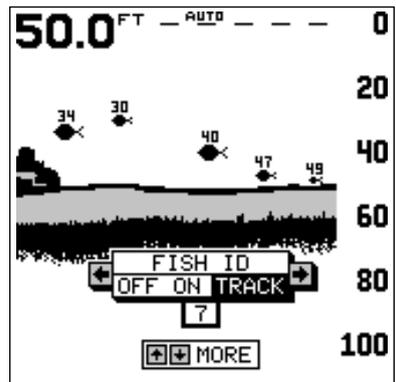
Remember, the Fish ID feature can't be used when the X-65 is in the manual mode. If you turn the Fish ID feature on when the X-65 is in manual, the microcomputer will turn the automatic feature on. If you turn automatic off when the Fish ID feature is on, the Fish ID feature will be turned off also.
