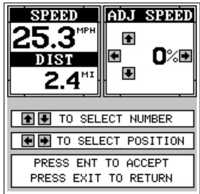
If the digital speed display is slower than your actual speed, add a positive percentage to make it read faster. If the digital speed display is faster, use a negative percentage to make it read slower. Use the arrow keys to change the speed, then press the ENT key. Press the EXIT key to erase this menu.
