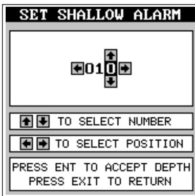
Press the ENT key to accept this setting. The X-65 returns to the alarms menu, showing a shallow depth of 10 feet. Now you can activate the alarm by highlighting the "Shallow Alm" label and pressing the right arrow key.
