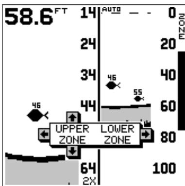
To adjust the top of the zone bar higher or lower, press the up or down arrow keys while the up and down arrows are surrounding the "Upper Zone" on the screen as shown above. To adjust the bottom of the zone bar, first press the right arrow key to move the arrows to the "Lower Zone" on the screen, then use the up or down arrow keys.
