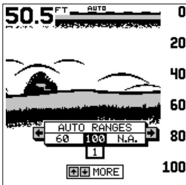
menu appears as shown at right. Press the left or right arrow keys to decrease or increase the range. The available ranges are 0-5, 10, 20, 30, 40, 60, 100, 150, 200, 300, 500, 800, and 1000 feet. After the desired range is displayed, press the EXIT key to erase the range menu.
